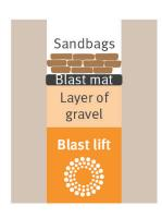
Once the charges are loaded, the 'blast lift' is covered by multiple layers to prevent flyrock and dust, as well as to decrease the impact of noise, overpressure and vibration from the site. These layers include:
