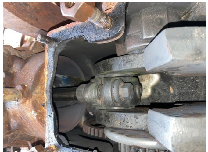
The babbit in the bottom of the crankcase
