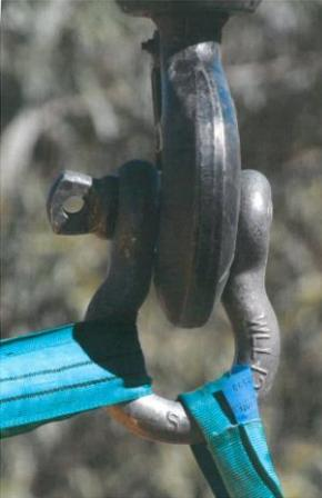
Following the introduction of soft slings, one disadvantage emerged - soft slings have no master link. If the risk of a sling detaching from the hook is to be as low as reasonably achievable, there must be a single attachment on the hook. This is easily accomplished by placing the soft slings onto a bow shackle and then placing a bow shackle on the hook with the pin of the bow shackle resting on the hook as shown in the image.
